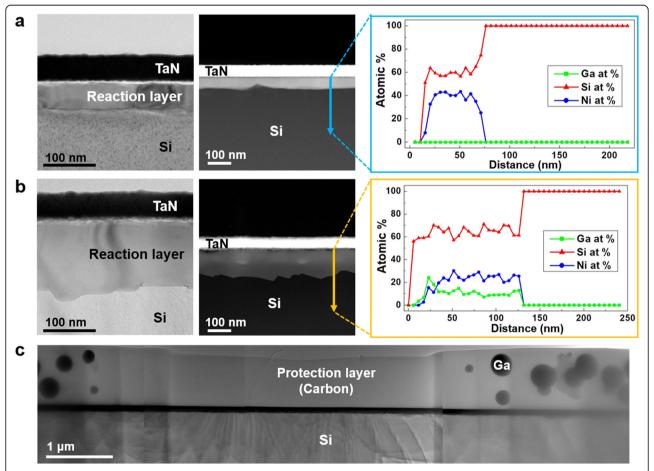
Fig. 2 The TEM/high-angle annular dark-field (HAADF)-scanning transmission electron microscopy (STEM) images and EDS line profile of the heat-treated TaN/Ni/Si thin-foil specimen prepared via (a) mechanical polishing and ion milling, and (b) FIB milling/EXLO, (c) The low-magnification TEM image of the TaN/Er/Si thin-foil specimen prepared via FIB milling/EXLO
