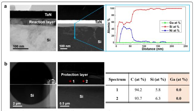
**Fig. 4** Result after the specimen attached to the FIB lift-out grid is subjected to Ar<sup>+</sup> ion milling. **a** The TEM/HAADF-STEM images and EDS line profile of the heat-treated graphene-encapsulated TaN/Ni/Si thin-foil specimen. **b** The TEM/HAADF-STEM images and chemical composition of the heat-treated graphene-encapsulated TaN/Er/Si thin-foil specimen
