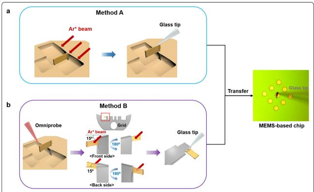
**Fig. 1** Schematic of the two different methods of  $Ar^+$  ion milling to remove  $Ga^+$  ions. **a** Performing  $Ar^+$  ion milling the lamella while leaving it inside the trench, **b** Performing  $Ar^+$  ion milling after taking the lamella out of the trench and attacing it to the lift-out grid
