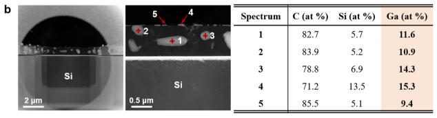
**Fig. 3** Results after the specimen in the trench is subjected to Ar<sup>+</sup> ion milling. **a** The HAADF-STEM image and the results of the EDS analysis of the heat-treated graphene-encapsulated TaN/Ni/Si thin-foil specimen. The Si K series, Ni K series, and Ga L series EDS mapping is shown in red, green, and orange, respectively. **b** The HAADF-STEM image and chemical composition of the heat-treated graphene-encapsulated TaN/Er/Si thin-foil specimen
